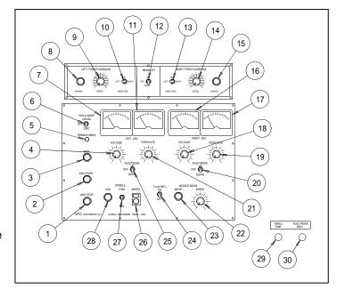
CROSS Mode moves the torch heads left and right over the roller or idler. At each end of the torch travel, the idler or roller turns briefly, overlapping the previous weld bead.
