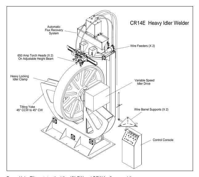
Power Yoke Tilt – rotates the idler 45° CW and CCW for flange welding.
